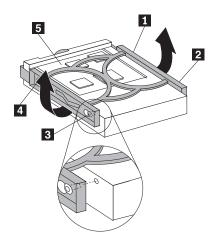
Figure 25. Installing the secondary hard disk drive into the bracket
